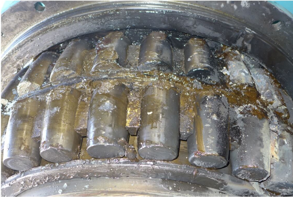
Figure 3: A Main Bearing (MB) failure, showing despite advances, concerns remain with high failure rates of this critical component in the drivetrain. Due to the MB's unique operating conditions, a considered investigation is required. [6].
