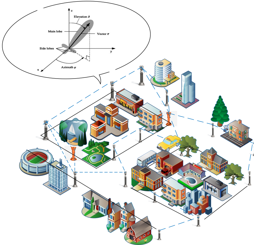
Figure 3.2: A sample mmWave integrated access and backhaul (IAB) network model with directional antenna.
