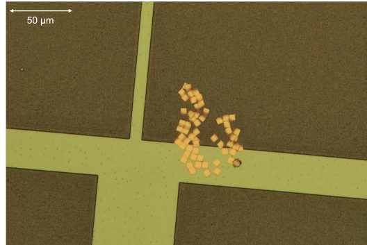
Figure 6.3: Clusters of drifted Au squares that appeared in subsequent fabrication stages, after the partial lift-off result. In total, only a small number of squares drifted across the chip, and usually not in clusters. However, there were occasional clusters or single squares that affixed to Py contacts, resulting in the rejection of otherwise well-fabricated contacts.
