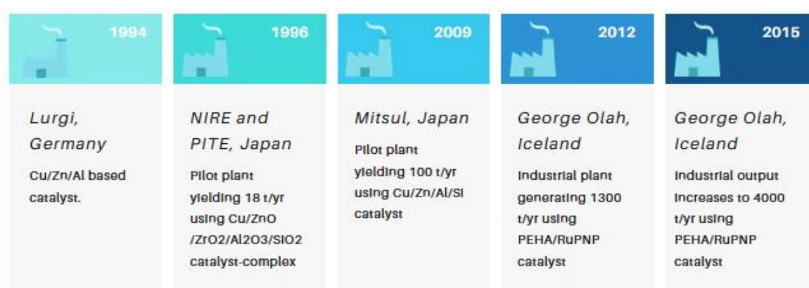
Figure 3. Technology progress of metal-catalyst mediated CO 2 hydrogenation to CH 3 OH, adapted from 63 .
