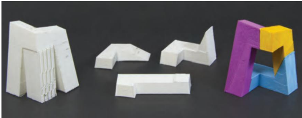
Fig. 2-3. Example of whole printed structure with support material (left), and pyramidal decomposition allowing parts to be printed without support material (right). Images from [26].
