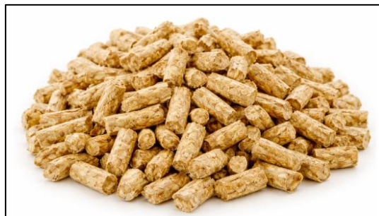
Figure 10: Wood Pellets as a Biomass-Derived Solid Fuel (image adapted from Wei, Mellin, Yang, Mefos, et al., 2013)
