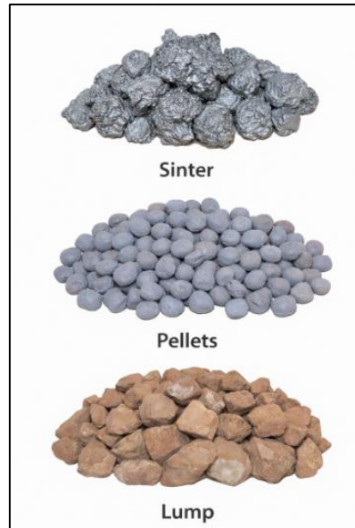
Figure 6: Physical Appearance of Iron-Bearing materials (Sinter, Pellets, and Lump Ore) (adapted from Geerdes et al., 2015)
