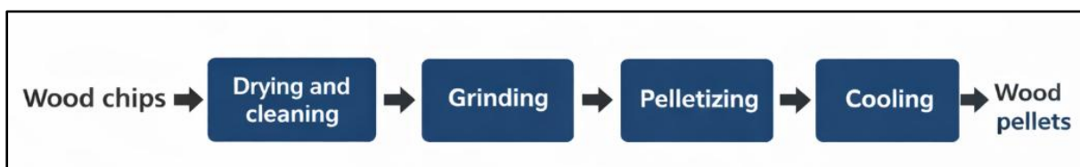
Figure 11: Process Flow of Wood Pellet Production (adapted from Wei, Mellin, Yang, Mefos, et al., 2013)
