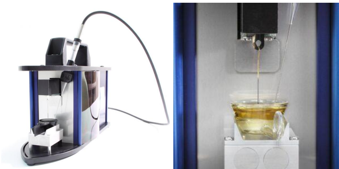
Figure 8: Left-hand side: The Kibron EZ Plus tensiometer used for high-precision surface tension measurements. Right-hand side: A close-up of the measurement stage, showing the sample dish beneath the sensor probe and a thermocouple monitoring temperature for accuracy.
