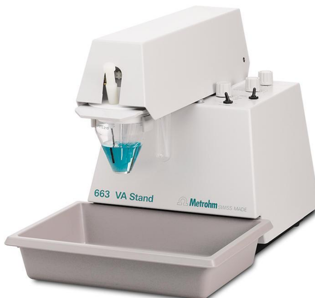
Figure 12: Metrohm 663 VA Stand used for voltammetric analysis of surfactant activity in sea surface microlayer (SML) samples.
