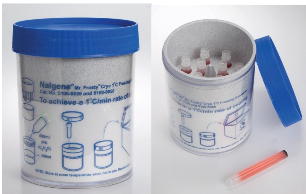
Figure 11: The image shows Mr. Frosty Freezing Container, used for freezing samples at a controlled rate of 1°C per minute using isopropanol (IPA).
