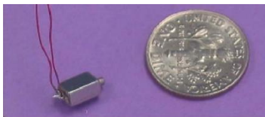
Figure 2.15: The size of microspeaker [3]
