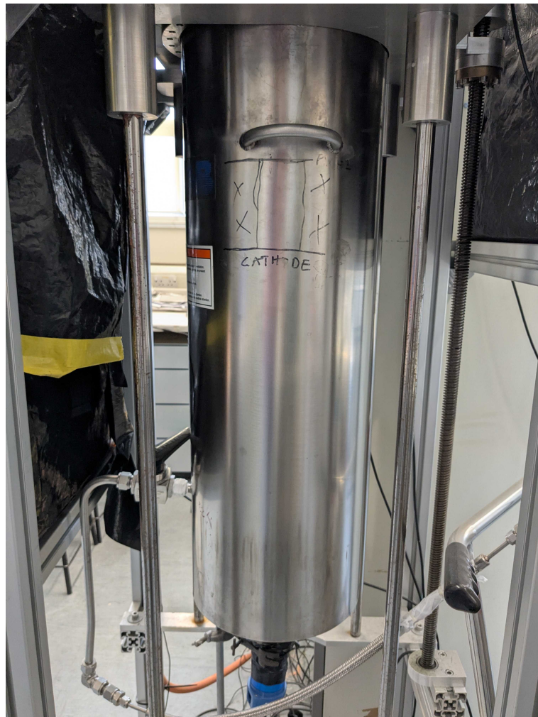
Figure 8.2: Picture of the STEEL dewar containing the LArTPC, indicated by the black drawing on the face of the dewar. It is a stainless steel cylinder 60 cm in height and 24 cm in diameter capable of containing 27.6 L of argon.
