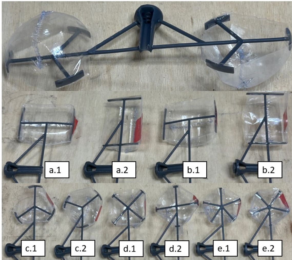
Figure 4.6: The top of the figure shows an AeroTail prototype, detailing all its components. Below are the various DI versions. Red tape is applied to the sides of each DI for enhanced visibility during experiments.
