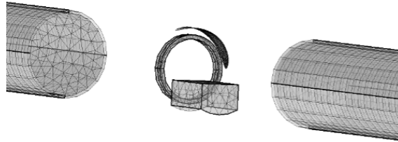
Figure 7.2: Robot as modelled in COMSOL, showing the geometry and mesh close to the robot/defect. The pipe next to the robot has been removed for improved visibility. The defect has been offset by 45° from the top of the pipe here as part of the analysis of the robot sensitivity in Section 7.1.2.
