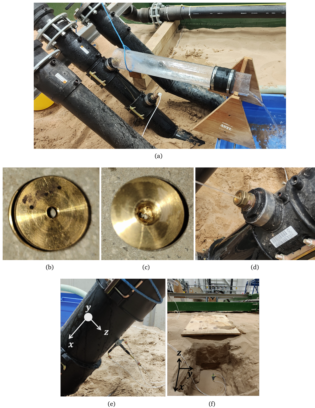
Figure 3.10: The experimental setup used to investigate the effect of different aperture shapes on the acoustic emission from leaks. (a) a wider view of the testing area, including the catchment system used; (b) the 3 mm leak insert; (c) the 2x2 mm leak insert; (d) the flow from the 3 mm leak when the catchment system has been removed; (e) the attachment method for the triaxial accelerometer; (f) the position of the accelerometer on the buried section of pipe when it is 4 m from the leak, the end of the pipe is just visible in the background of this photograph.
