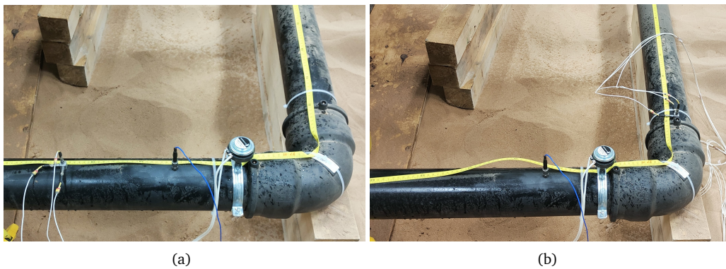
Figure 4.31: Location of shaker and accelerometers for measurements across a 90 degree join, showing (a) the positions of the shaker and accelerometers for measurements along a straight pipe section and (b) around the corner, with the monoaxial accelerometer acting as a reference.
