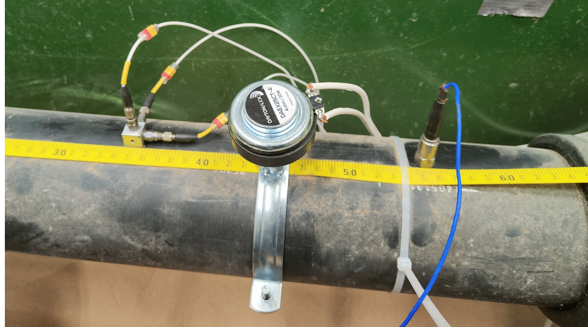
Figure 4.18: The shaker and accelerometer setup on the HDPE pipe used to measure the acoustic attenuation.
