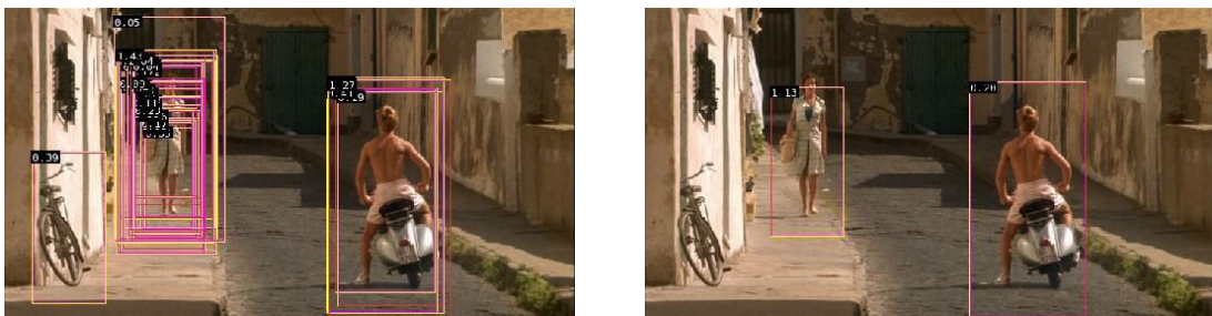
Figure 4.5 Merging HOG detections by multi-scale object localisation
