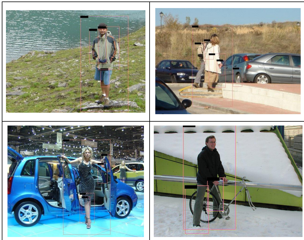
Figure 4.7 Examples of the original HOG detections with overlapping detection windows on body parts
