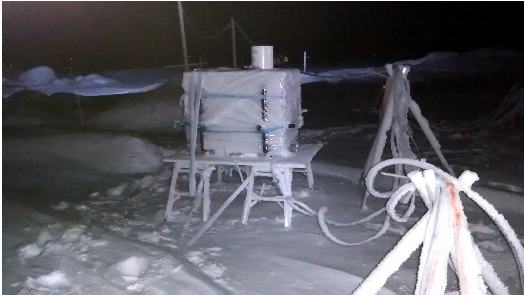
Figure 2.13 University of Leeds Halo Doppler lidar in the Met City. Photograph taken on November 2, 2019 when the Lidar had to be wrapped up in insulating panels and plastic sheet to get it warm enough to restart after a long power cut. Credits: I. Brooks.
