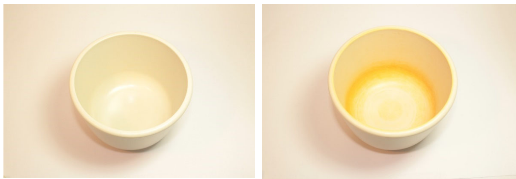
Figure 3.3 Example of images shown to respondents - bowl 9, which had been tested with baked beans on the heavy use regime after 1 cycle (left) and 28 cycles (right).
