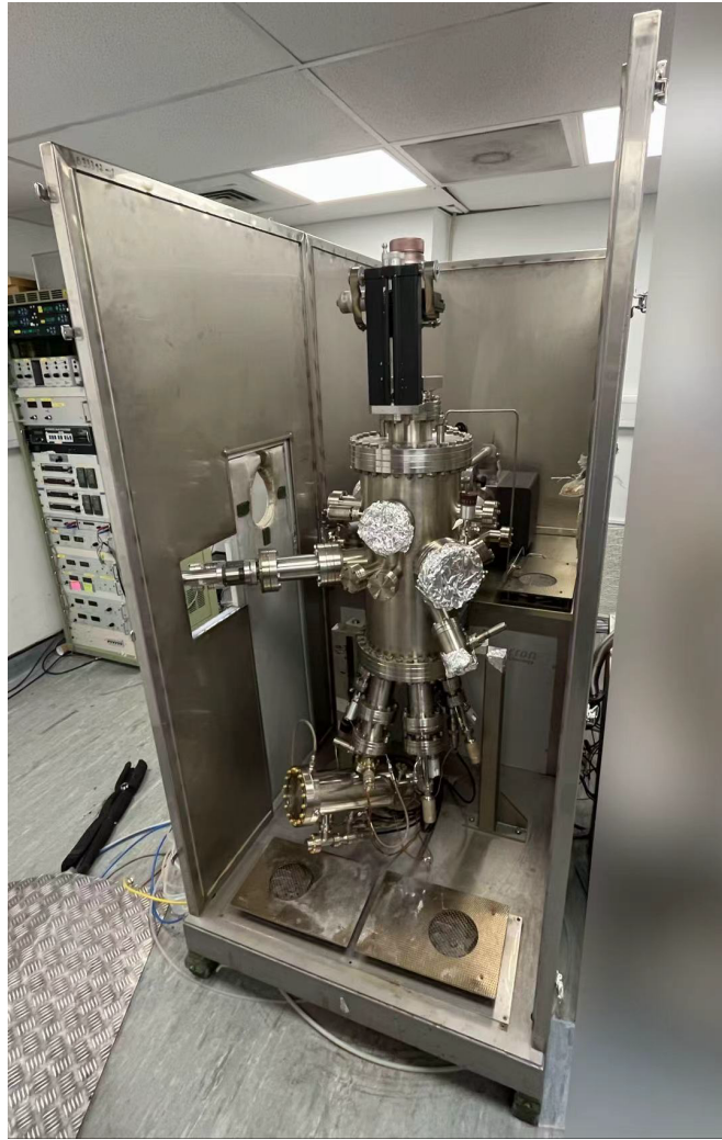
Figure 3.13: Bake-out preparation of MBE system
