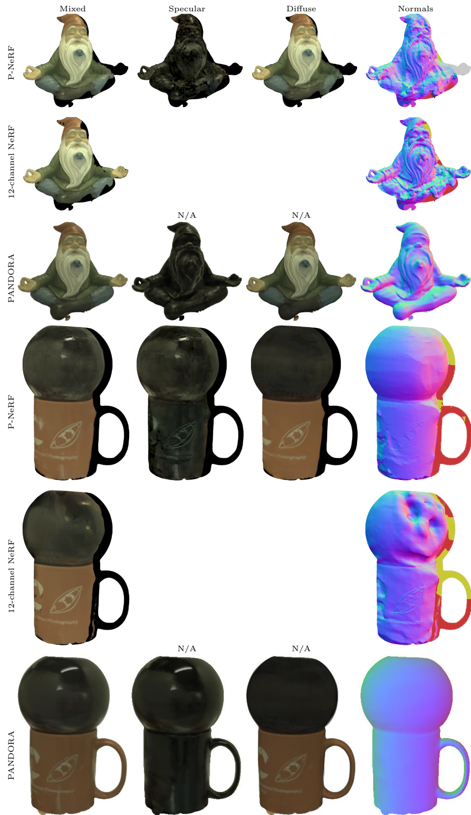
Figure 4.10. Reflectance decomposition and geometry estimation of (real-world) gnome and vase data.
