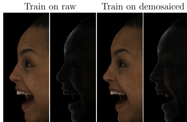
Figure 5.16. Demosaicing ablation: On the left we show diffuse and specular radiance for our method. On the right we show an ablation where we first demosaic and then train our method on all channels. Zoom to see blurring artefacts.
