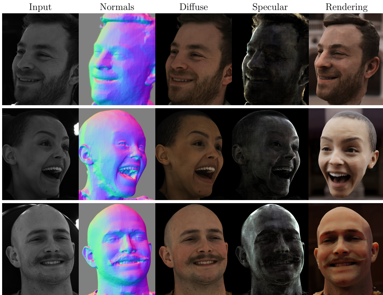
Figure 5.13. Three facial subjects with different skin-tones . Columns: (1) raw CPFA view, (2) predicted surface normals, (3) diffuse radiance, (4) specular radiance, and (5) mesh re-rendered with the recovered material maps under a distinct HDR light probe for each subject [81]. All images are tonemapped for display.
