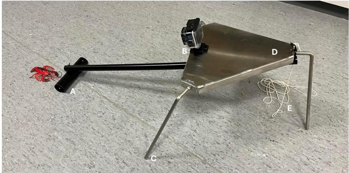
Figure 3.1. Final construction of the CrayCam system with. A) Removable PVC bait arm, B) GoPro Hero10 with action mount, C) removable and posable legs, D) Base plate, E) rope for attachment to bank
