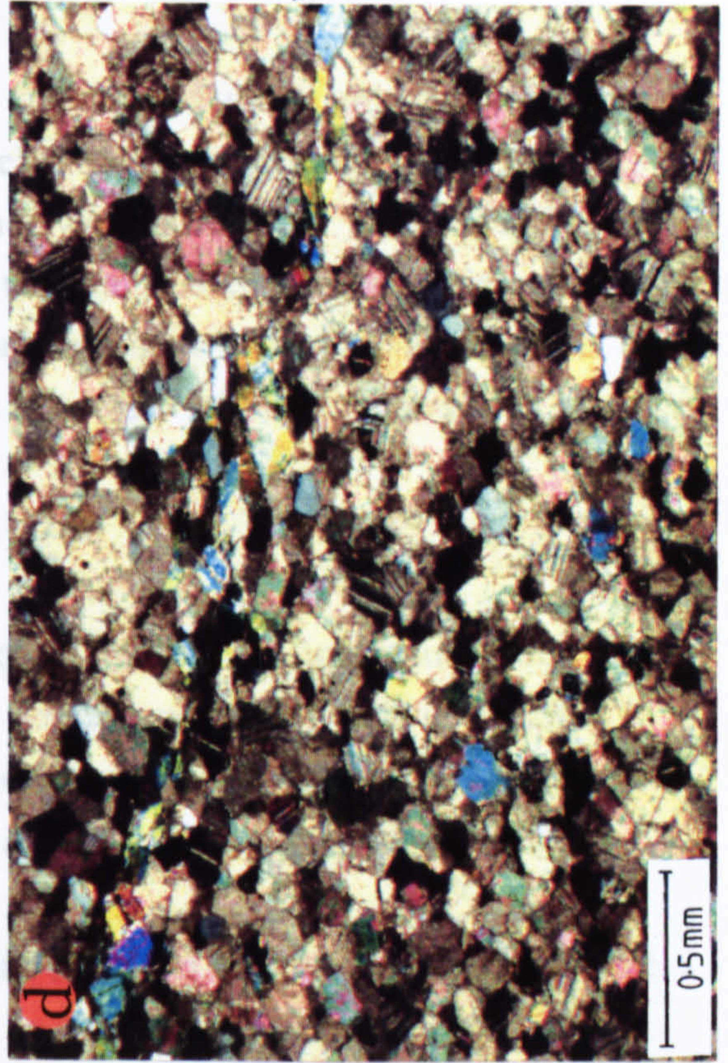
Delimiting carbonate is observed within the quartz domains and these are up to 1mm in size. A dark opaque phase is also present.
