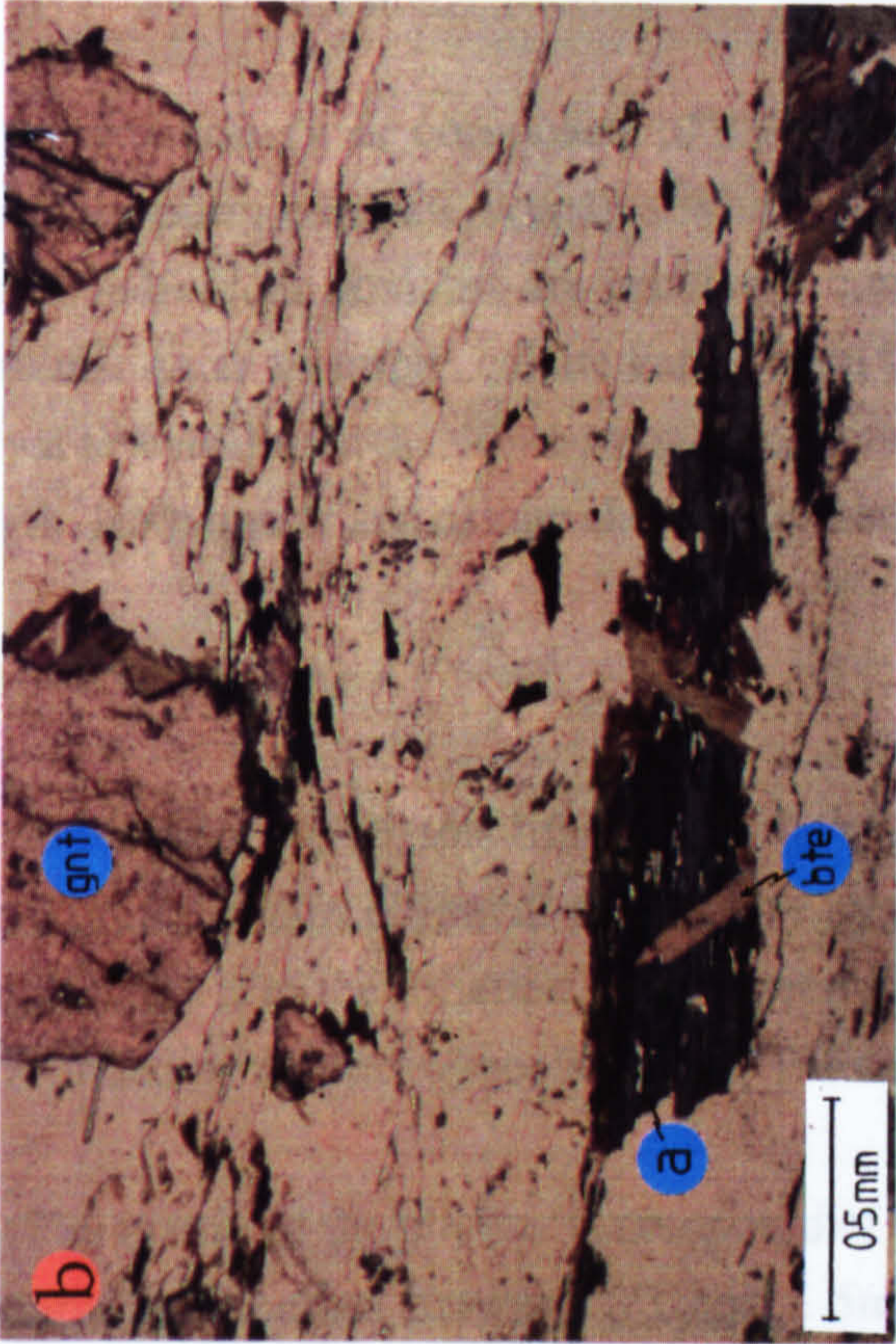
Delimiting carbonate is observed within the quartz domains and these are up to 1mm in size. A dark opaque phase is also present.
