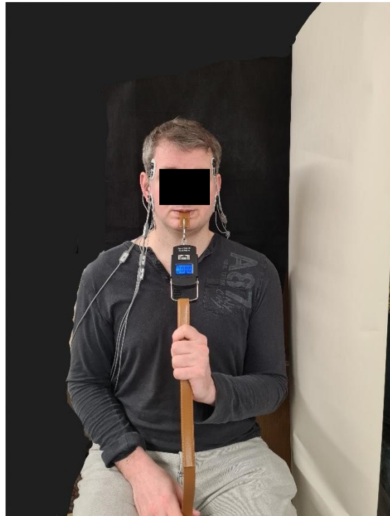
Figure 4.09 Image of participant biting on a piece of leather belt at the incisors whilst pulling anteriorly and downward.
