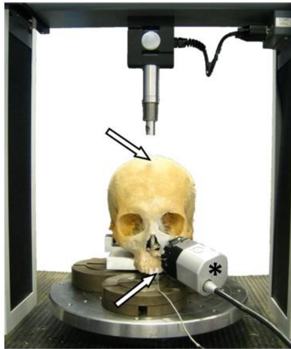
Fig 3.01: Image of the experimental set up for strain measurement; vertical compressive load applied to the calvarium (upper arrow) simulating a left central incisor bite (lower arrow). The asterisk shows the DSPI sensor attached to the infraorbital region (Toro-Ibacache et al., 2016, p. 72, fig 1).
