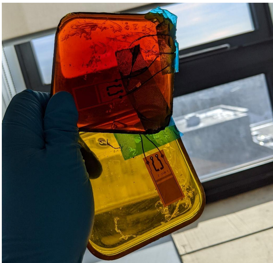
Figure 5.5 – TGpAP/44'DDS cured using a 160 °C dwell where the top resin underwent a ramp at 1 °C min -1 , whereas the bottom resin underwent a ramp at 0.5 °C min -1 .
