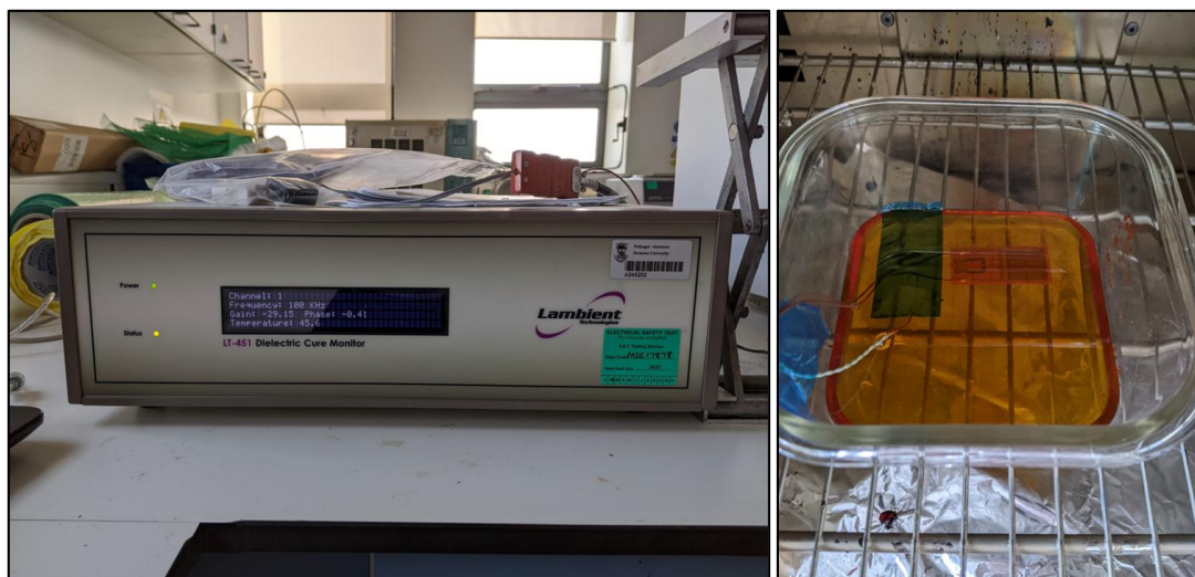
Figure 3.10 – An image of the Lambient LT-451 Dielectric Cure Monitor equipment and resin cast onto a Mini-Varicon sensor with a K-type thermocouple.
