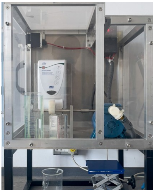
Figure 3.1: Digital photograph of the foam-forming apparatus used in this study. This equipment was designed and built by Ward-O'Brien et al. 41
