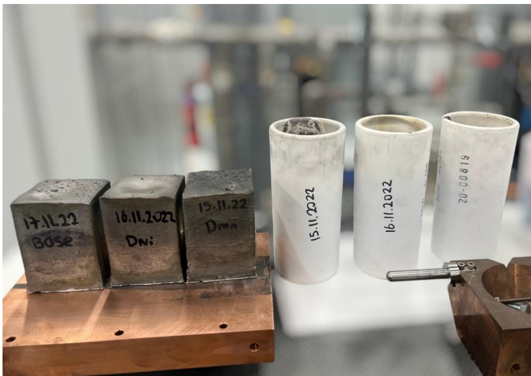
Figure 3.3 The three 5000 g ingots cast via VIM (left) along with the one-shot liners which were dried and conditioned by applying a low induction power that was increased gradually until the alloys were melted (right).
