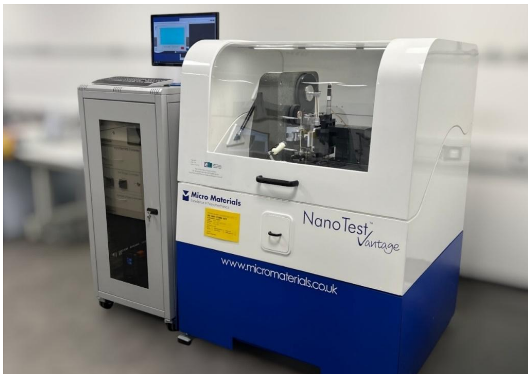
Figure 3.19 NanoTest Vantage system used to perform depth versus load hysteresis nanoindentation testing.
