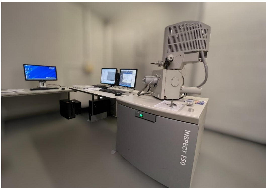
Figure 3.13 Inspect F50 scanning electron microscope used to acquire high resolution images of the deformed microstructure.
