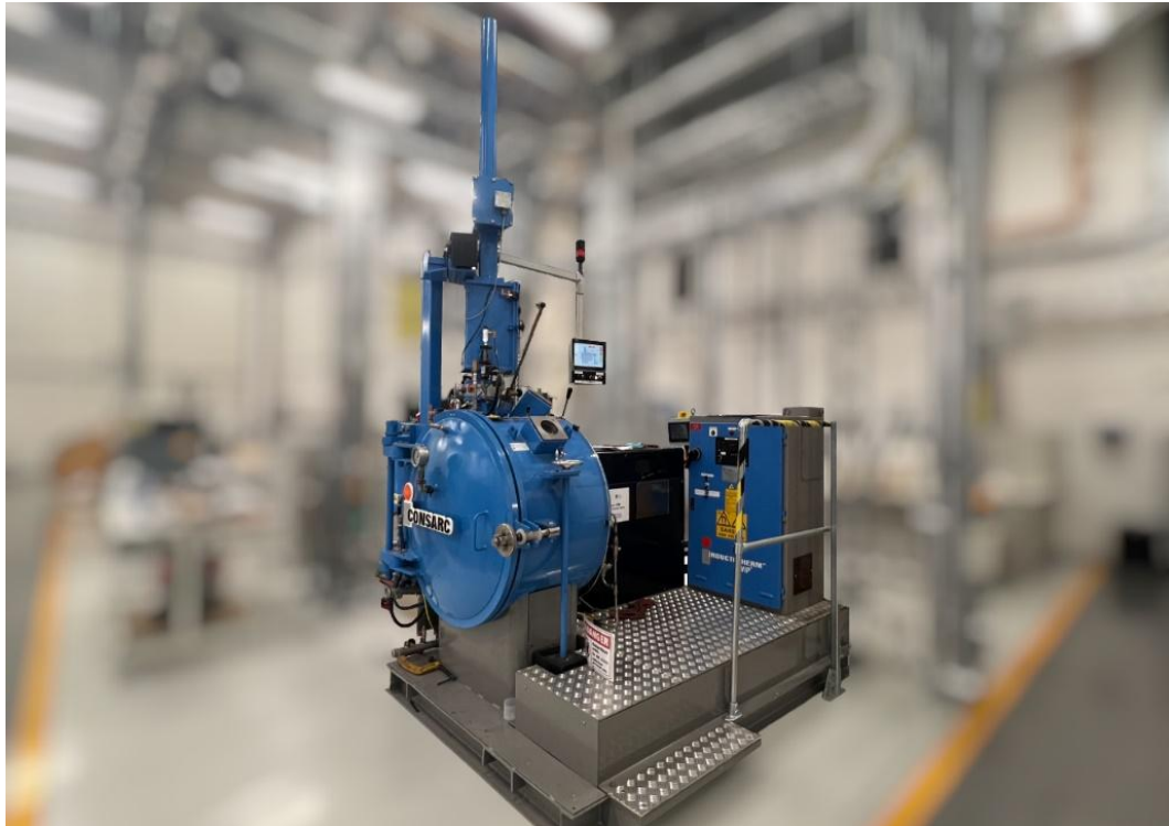
Figure 3.2 Vacuum induction melting furnace used for casting of the three homogeneous 5000 g ingots, located at Royce Discovery Centre.
