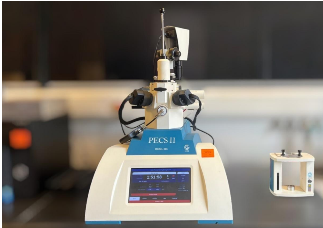
Figure 3.14 Automated argon ion polishing system used to accomplish damage-free surfaces securing successful EBSD analysis; the loading dock on the right-hand side is used to adjust the height of the mounted specimen before transferring it into the system.
