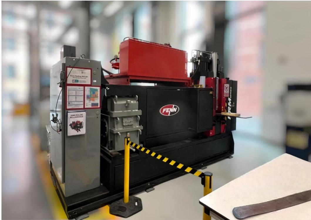
Figure 3.4 Hot rolling mill used to roll the three ingots into plates, reducing their thickness to 12 mm, where one of these plates appears at the bottom right corner.
