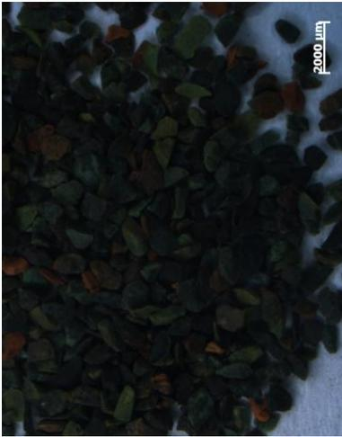
Figure 5.16: Fresh copper oxide
