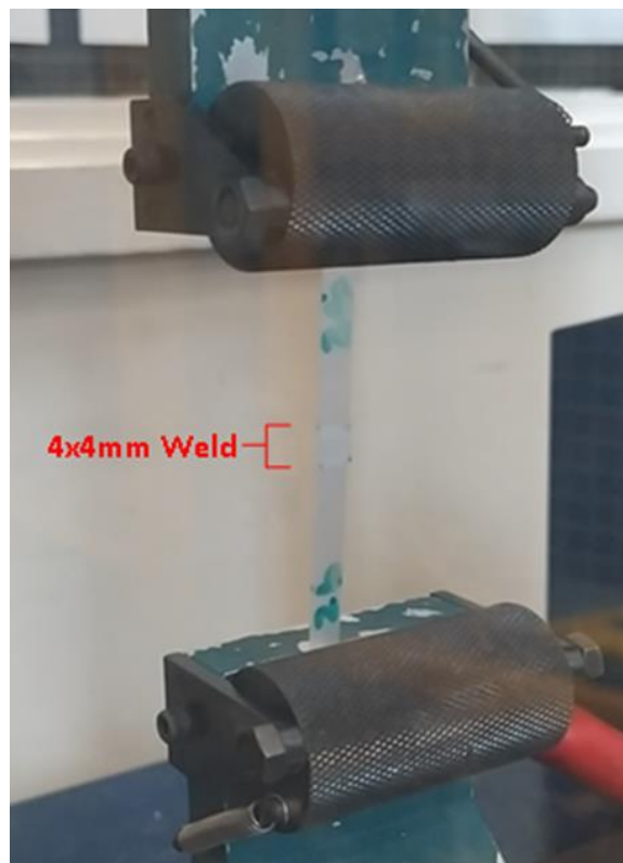
Figure 3.8 Clamp arrangement for the Hounsfield tensile tester with an ultrasonically welded PVDF strip product held in position, under tension, ready for mechanical testing.
