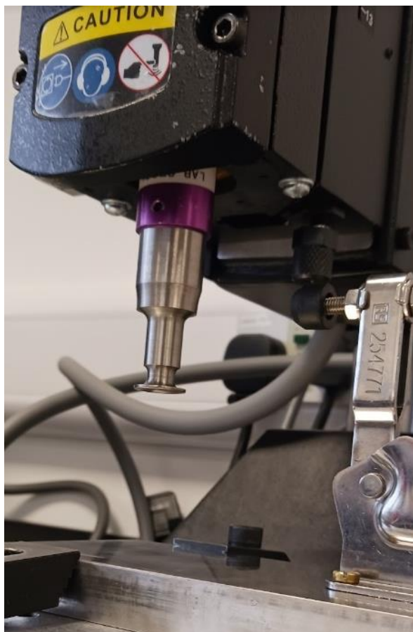
Figure 3.12 Branson 2000X ultrasonic welder with the booster removed, ultrasonic welder pressure gauge, the 0.75x gain purple booster with the welding horn attached, the welding horn in position.
