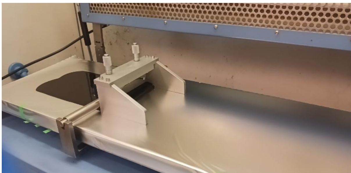
Figure 3.13 Slurry casting of NMC622 slurry on aluminium foil using a doctor blade.
