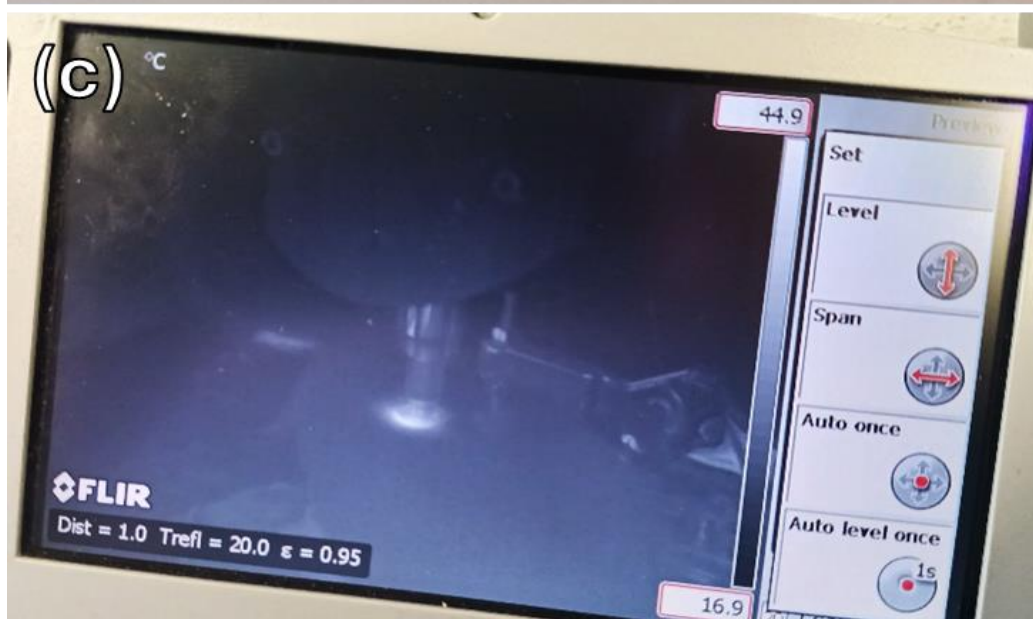
Figure 5.15 Images taken during ultrasonic calendering of NMC cathodes. (a) visual spectrum image of set-up (b) FLIR infra-red thermal image prior to activation (c) FLIR infra-red thermal image during actuation of the ultrasonic calendering. The cathode shows the peak temperature of 44.9 °C during actuation. The welding horn does not match this temperature rise.
