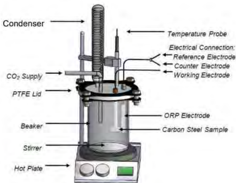
Figure 66 Typical set-up for static corrosion test (also the same for scaling tests)
