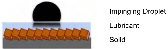
Figure 83 Schematic of SLIPS configuration. Impinging droplet (d), Lubricant (l) and solid (s)
