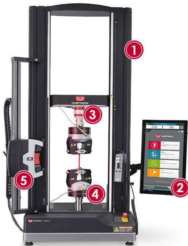
Figure 3.10 Tensile testing machine wherein 1: Load frame, 2: Software, 3: Load cell, 4: Grip to hold the sample tightly, and 5: Strain measurement [129]
