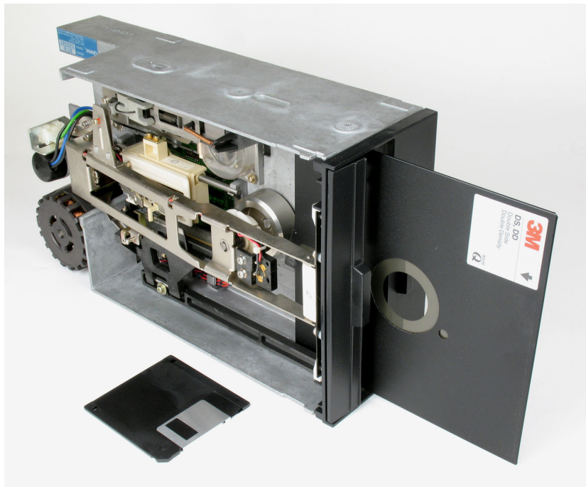
FIGURE A-1.6. Floppy disk drive for 8 inch floppy disks, introduced in 1978, next to a 3\frac{1}{2} inch diskette from 1984 (Image: Public domain).
