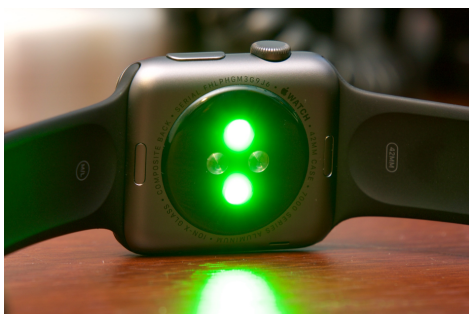
Figure 3.3: Sample of a smart-watch with PPG sensor emitting green light, ready to measure heart rate from Healthcare Digital 1 .
