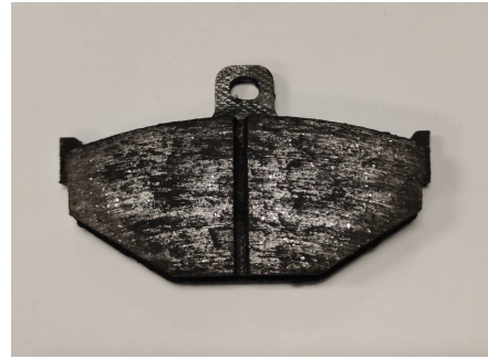
(b) Image of Lotus Elise S1 brake pad cut to fit inside brake calliper
