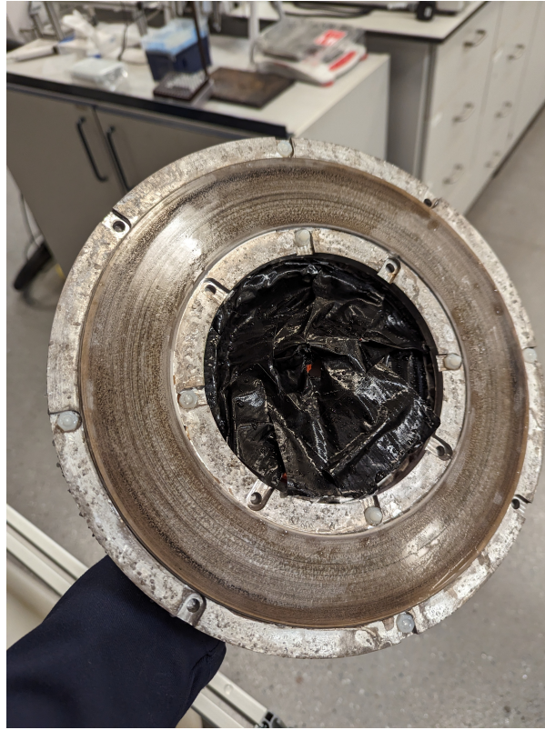
Figure 3.20: Three-piece rotor with nylon screws and tape for corrosion cabinet
