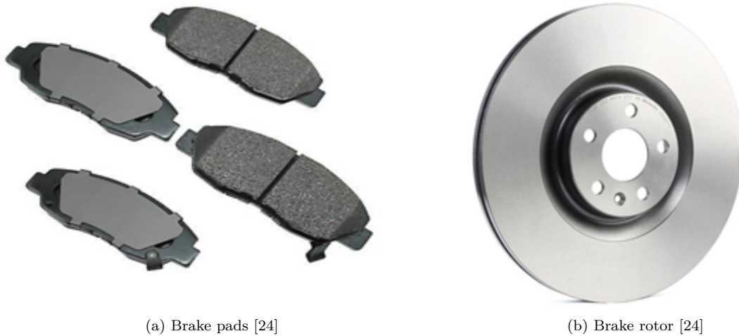
Figure 2.2: Brake friction pair
