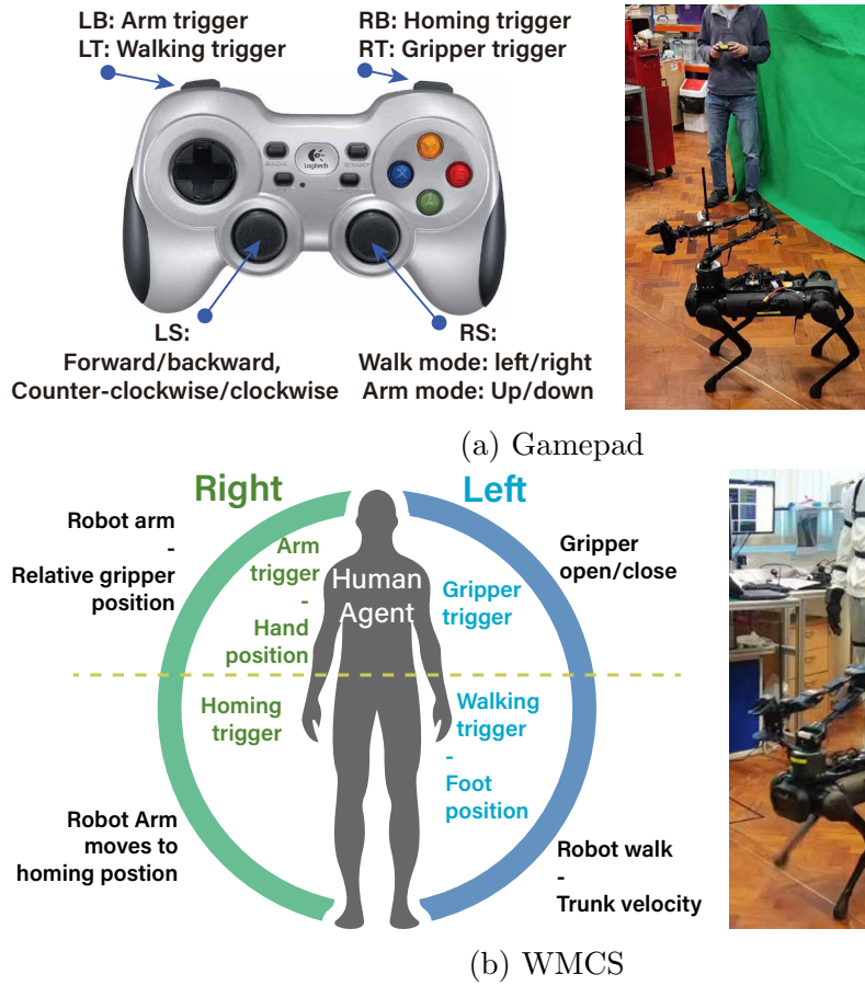
Figure 3.5: Details of mapping from interfaces to trigger and argument strategies, and experiment operation example: (a) gamepad, (b) WMCS. For the WMCS, each trigger is active by the user closing his/her hand.
