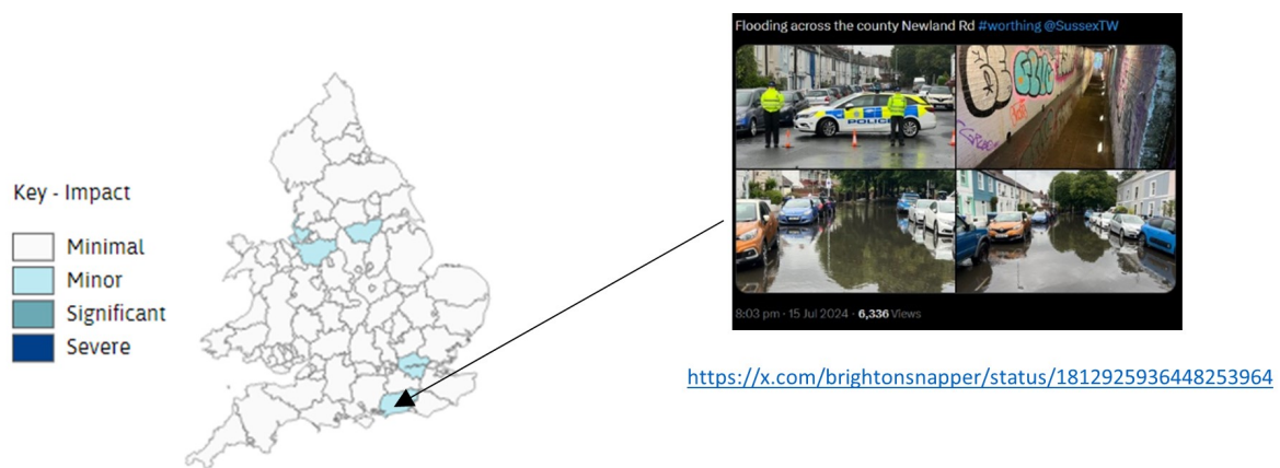
Figure 6.1: Left An example of a county scale map of reported SWF, with their associated severity level, for 15th July 2024 (impacts may have been reported at any time during the day). Left An image extracted from a post on https://x.com/ giving evidence of minor surface water flooding in Worthing, Sussex. This SWF event report is scaled up to the county level to produce the mapped impact level shown (left).
