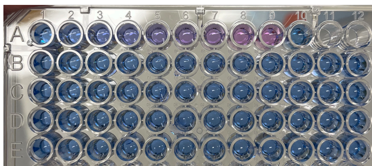
Figure 4.6: Standard Curve for DMMB Assay. (A) Standard curve created with serial dilution of Chondroitin Sulphate and absorbance read at 530 nm, alongside samples. (B) Image of plate with standard curve in row A and samples in rows B-E.
