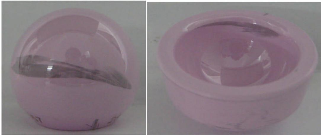
**Figure 3.6: The wear stripe on the ceramic femoral head and the rim wear of the acetabular cup formed after testing under microseparation conditions. The wear areas were marked with pencil rubbing for clarity (the grey colour was not due to the wear test).**
