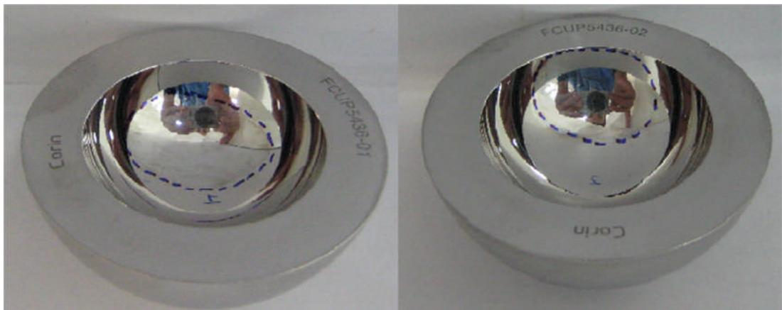
**Figure 6.4: Photographs of the 36mm inner diameter acetabular cups showing the wear area (within dotted line) under standard conditions with 45° inclination angle (left) and the wear area under steep inclination angle (right). Under steep inclination angle the wear area approached the rim of the acetabular cup but it did not intersect with the rim after 3 million cycles of test under standard gait conditions.**
