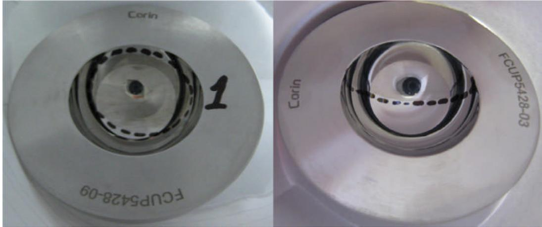
**Figure 6.5: Photographs of the 28mm inner diameter acetabular cups showing the wear area (within dotted line) under standard conditions with 45° inclination angle (left) and the wear area under steep inclination angle (right). Under steep inclination angle the wear area intersected with the rim of the acetabular cup.**
