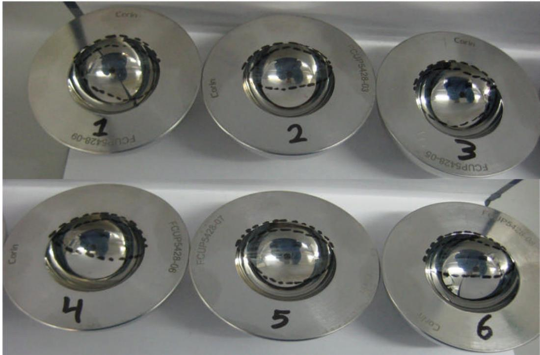
**Figure 4.14: Images of the 6 acetabular cups after 6 million cycles of testing. Ink marking show two distinct wear areas; a smooth wear area at the bottom with a rougher wear area adjacent to the rim of the acetabular cup.**
