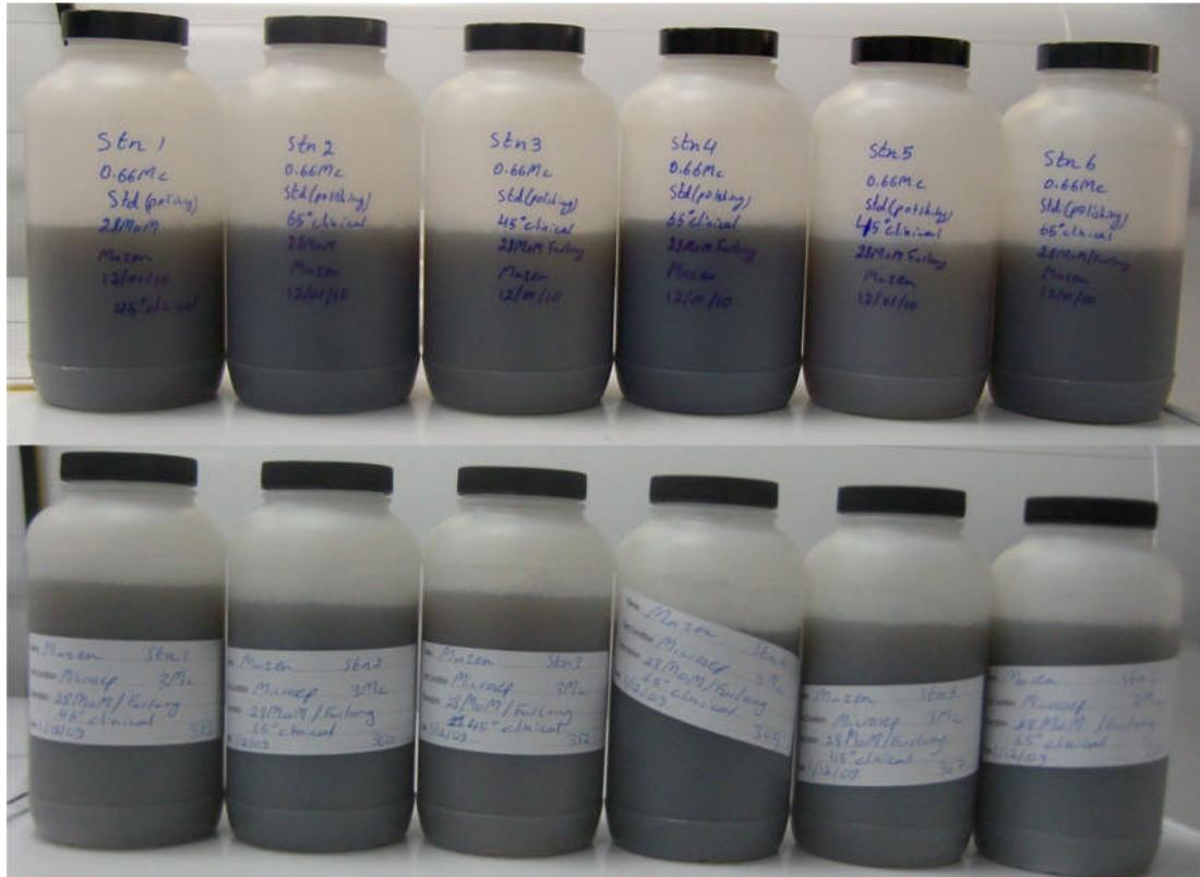
**Figure 4.7: Serum colour for all stations at 0.66 million cycles of test (top) and 3 million cycles of test (bottom) under microseparation conditions. Stations 1, 3 and 5 had the cups inclined at 45° and 2, 4 and 6 had the cups inclined at 65°.**
