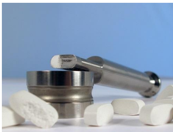
Figure 1-3. Pharmaceutical powder mass adhered to the upper punch 24
