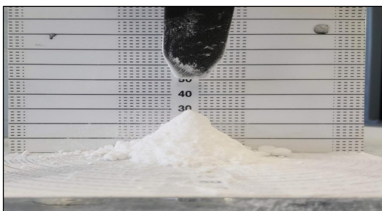
Figure 4-6. Angle of repose test on d-mannitol
