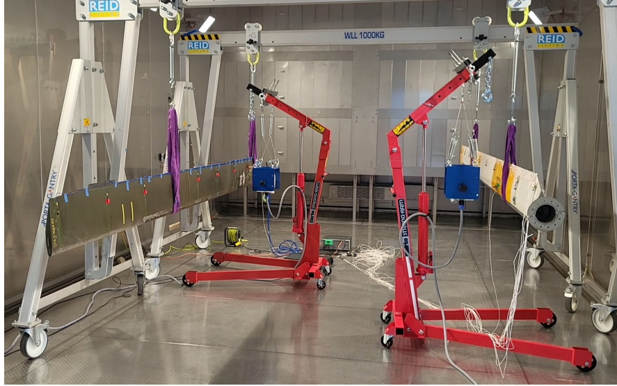
FIGURE 5.6: The experimental setup to perform modal testing on a metal (right) and composite (left) blade simultaneously.
