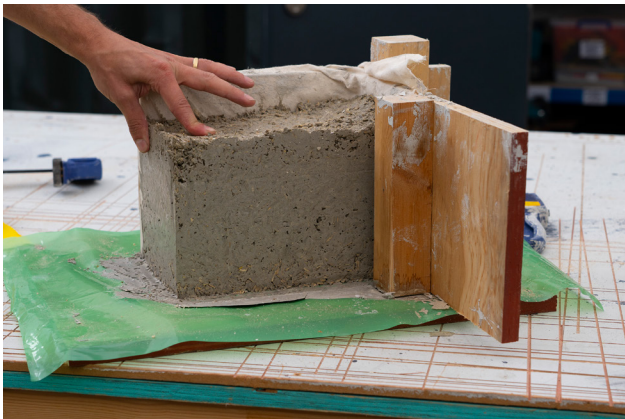
Figure 54 - Hempcrete Block Mixes - increased lime and sand
