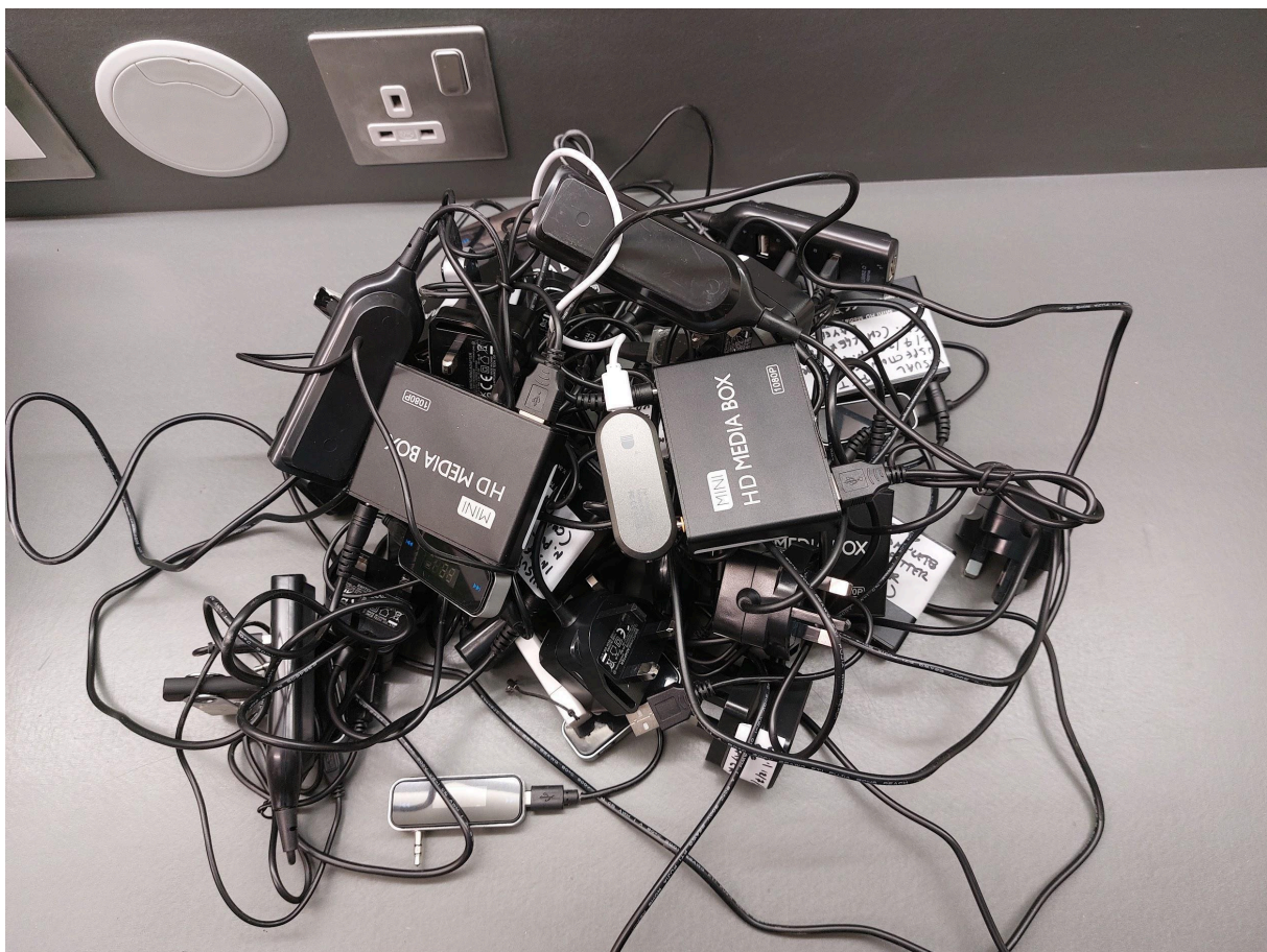
Figure 38: Pile of broadcasting devices used for the installation, including media players, fm transmitters, and usb splitters.
