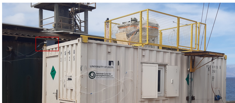
Figure 5.4: LOPAP inlet (framed by the red box) on top of the FAGE container at the CVAO during the February 2023 campaign.
