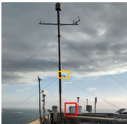
Figure 3.2: The NO x inlet (highlighted in orange) on the side of the 10 m tower and the NO x inlet box (highlighted in red) on the roof of the KCG BAPS.
