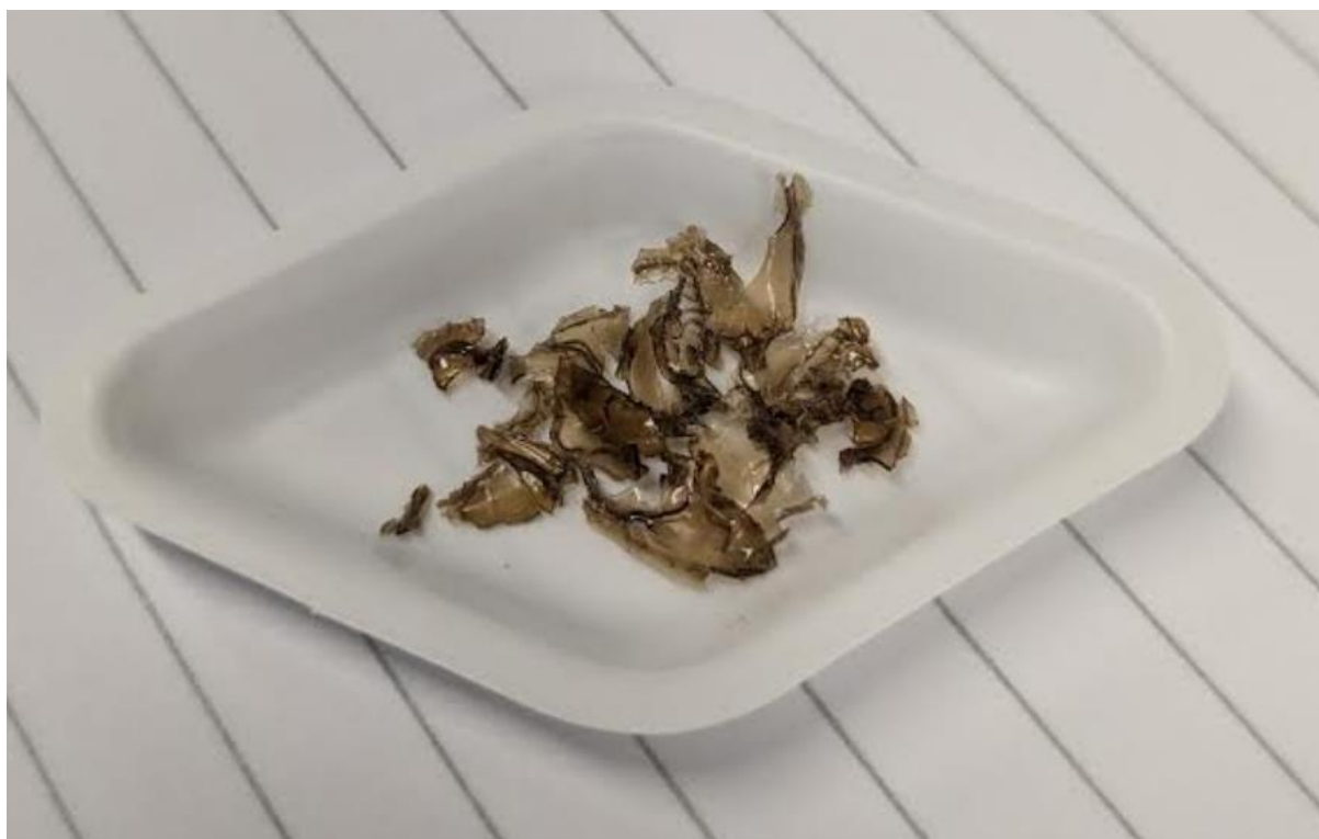
Figure S4. Fragments of (\text{H}_2\text{BNH}^n\text{Pr})_n film obtained by evaporation of the toluene reaction solvent used in the dehydropolymerisation of \text{H}_3\text{B}\cdot\text{NH}_2^n\text{Pr} with 8 (0.5 mol%, activated with 0.05 \text{ mol dm}^{-3} of \text{NH}_2\text{Me} ).
