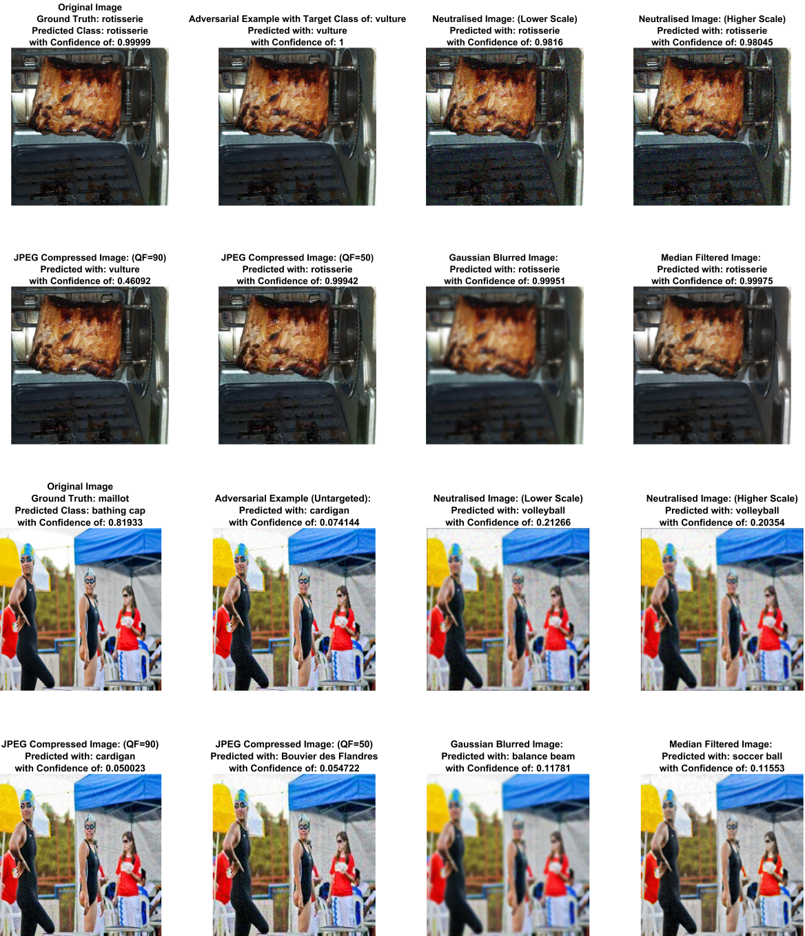
Figure 3.12: Examples of using different pre-processing methods for the defence of adversarial examples (PGD attack).
