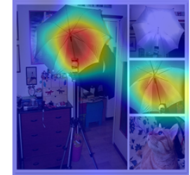
Figure 4.8: Feature Visualisation Comparison between ResNet-101 and Hybrid WSN-ResNet-101. Set(1): Clean image correctly classified by ResNet-101 and the corresponding Grad-CAM; Set(2): AE misclassified by ResNet-101 and the Grad-CAM of AE; Set(3): Same AE correctly classified by WSN-ResNet-101 and the Grad-CAM showing its attention focus by the hybrid network.
