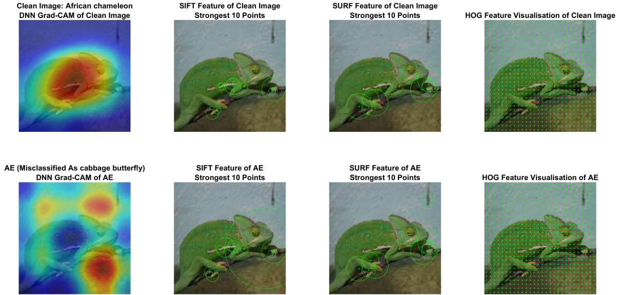
Figure 4.1: Visualisation of different feature maps extracted from a clean image and its corresponding adversarial example. DNN feature maps are visualised using Grad-CAM to highlight class-discriminative regions. SIFT and SURF maps display the ten strongest keypoints, respectively, while HOG maps are shown by superimposing oriented gradient vectors to illustrate local edge orientation patterns.
