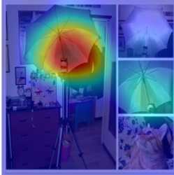
Figure 4.8: Feature Visualisation Comparison between ResNet-101 and Hybrid WSN-ResNet-101. Set(1): Clean image correctly classified by ResNet-101 and the corresponding Grad-CAM; Set(2): AE misclassified by ResNet-101 and the Grad-CAM of AE; Set(3): Same AE correctly classified by WSN-ResNet-101 and the Grad-CAM showing its attention focus by the hybrid network.
