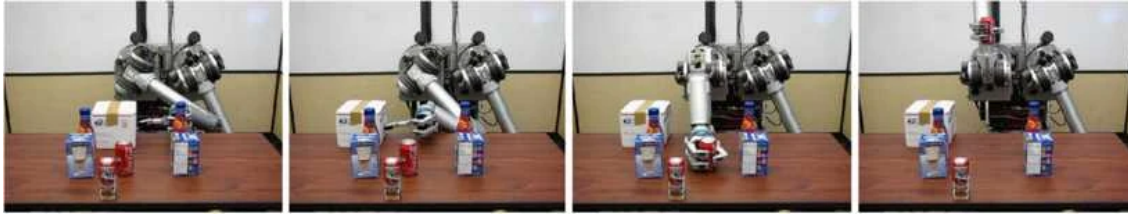
Figure 2.3: The robotic arm attempts to push the large box aside to grasp a red can positioned behind it [21] (figures, from left to right, represent sequential frame segments of the robot manipulation).
