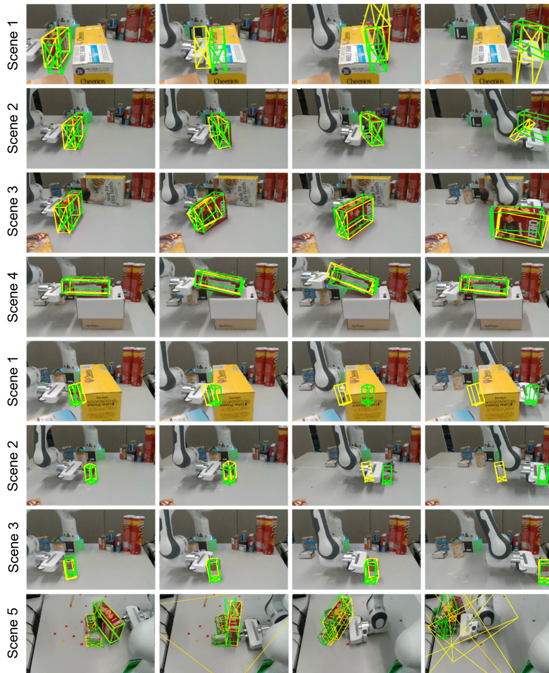
Figure 4.3: The estimated multi-objects poses of the method (PBPF-V) are shown as a green wireframe box. The poses from a vision-only system (DOPE) are shown as a yellow wireframe box.
