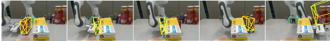
Figure 2.4: The goal of the task shown in the image is to track the red box being manipulated by the robot. The estimated pose of this red box is overlaid as a wireframe onto the image, during a push by a robot. Images show the estimated pose by a learning-based pose estimation system, DOPE [36] (figures, from left to right, represent sequential frame segments of the robot manipulation).
