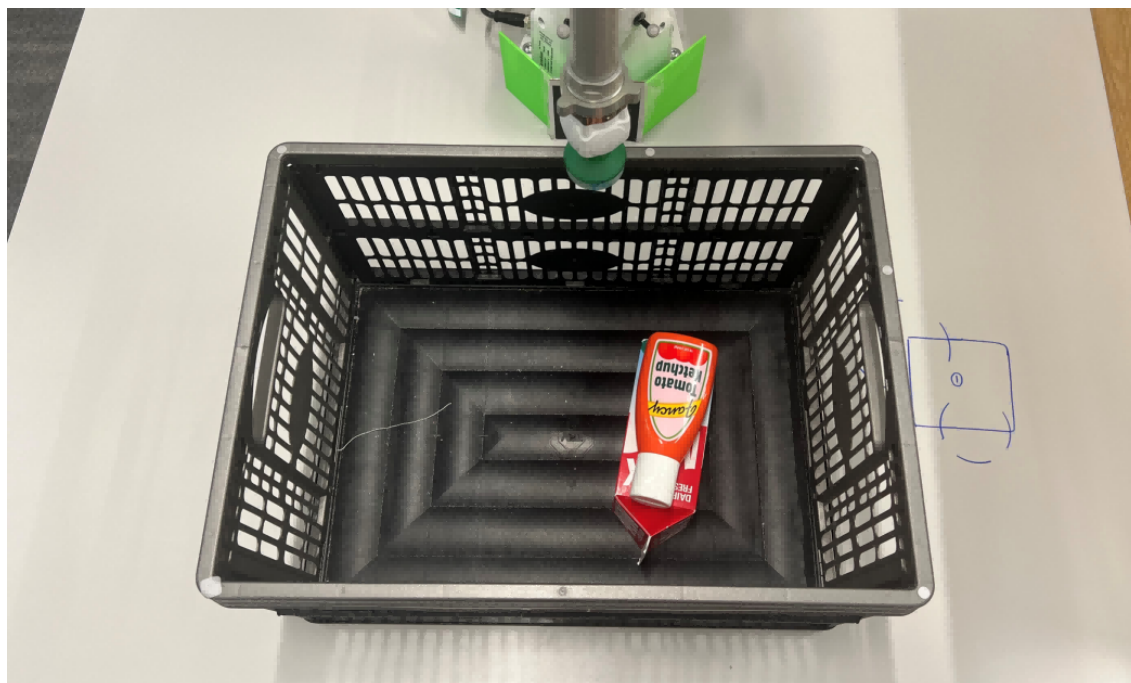
Figure A.1: Stacked objects in a basket scene. As shown in the figure, the ketchup is placed on top of the milk, and the camera looks down into the basket from above. The milk is occluded by the ketchup, making it impossible for the system to determine the milk's initial 6D pose.
