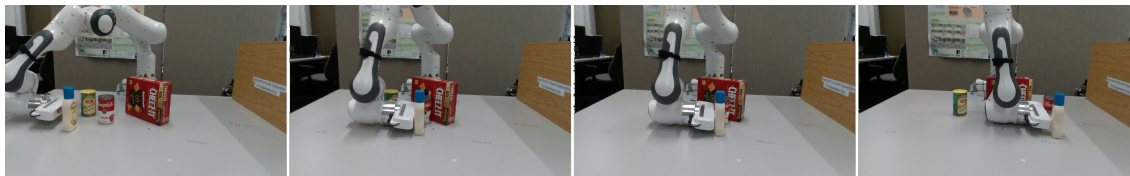
Figure 1.2: Robot is pushing 4 objects. The images are from the tracking camera, showing frequent occlusions among objects and by the robot arm.
