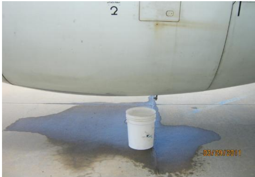
Figure 2.10: Fuel leaking due to the sealing problem. Reproduced from [73]
