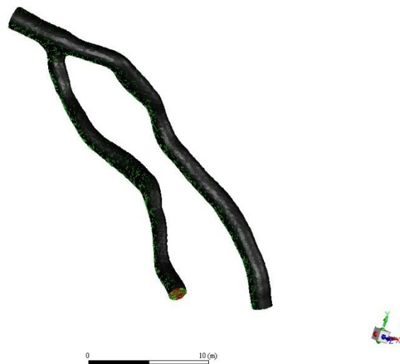
Figure 6.20. (Top) Volume mesh of the fluid domain and (Bottom) An example of a CFD simulation with pressure boundary conditions performed on this bifurcating model.
