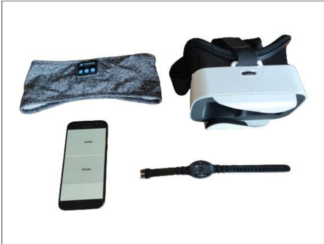
Figure 2.1 Equipment used; Sleep headband with integrated wireless headphones, headset to hold phone for visual stimulation mode, smartphone with hBET app loaded, Motionwatch 8 actigraph watch.
