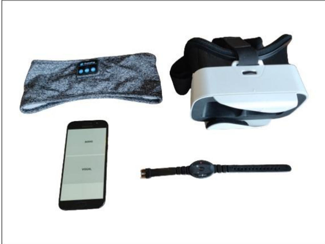
Figure 3.1 Equipment used by participants. Headband with integrated Bluetooth speakers for audio stimulation mode, headset to hold phone for visual stimulation mode, smartphone displaying home-based Brainwave Entrainment Technology application menu and MotionWatch.
