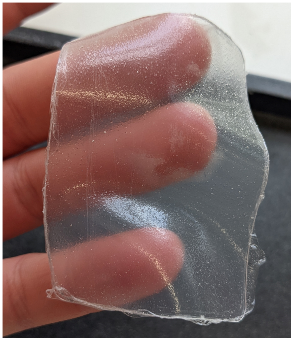
Figure 4.5: 1 mm thick upper layer made out of Silskin 10 special Effects RTV silicone (MB Fibreglass).
