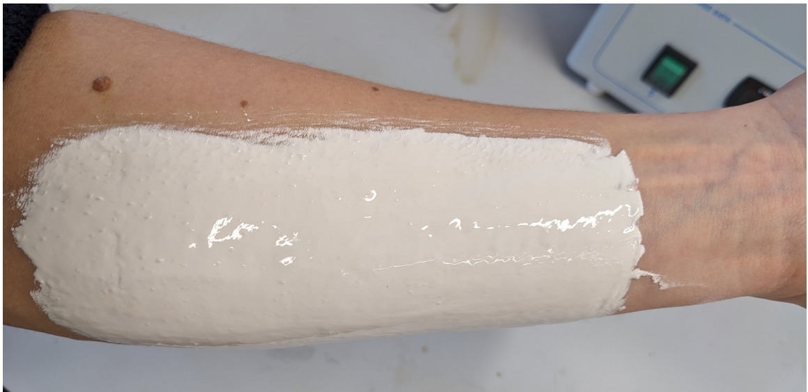
Figure 4.7: Method used for obtaining a replica of volar forearm texture using SILFLO.
