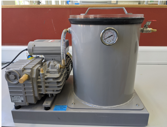
Figure 4.4: Degasser used to remove air bubbles from silicones.
