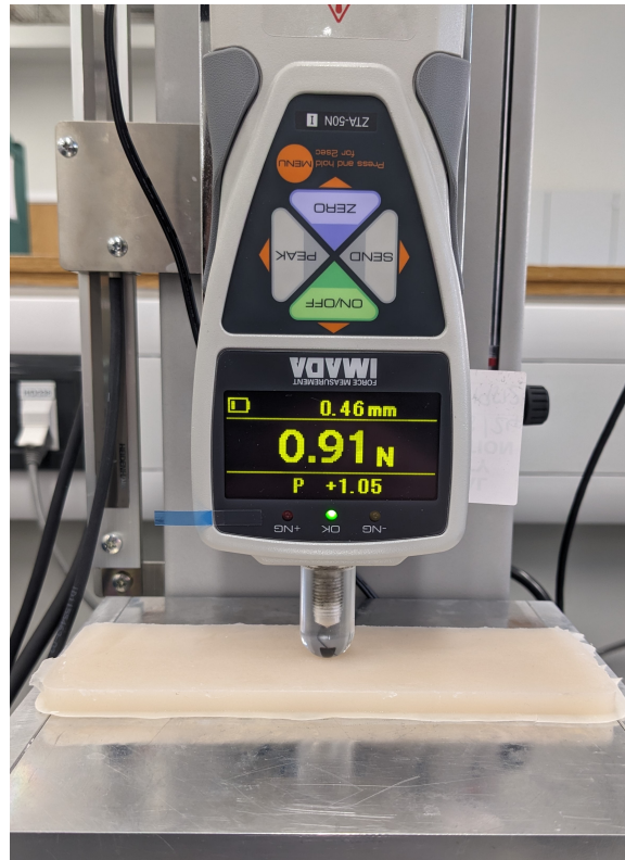
Figure 4.15: Force gauge set-up used for the indentation tests.
