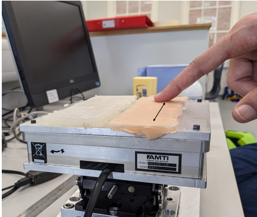
Figure 5.4: Human finger sliding against a synthetic skin test-bed for friction measurements with arrow showing the direction of sliding.
