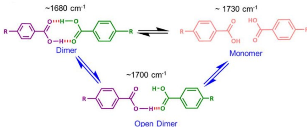
Figure 8.13 The FTIR characteristic spectra change of dynamic hydrogen bond change. Reproduced from [12]
