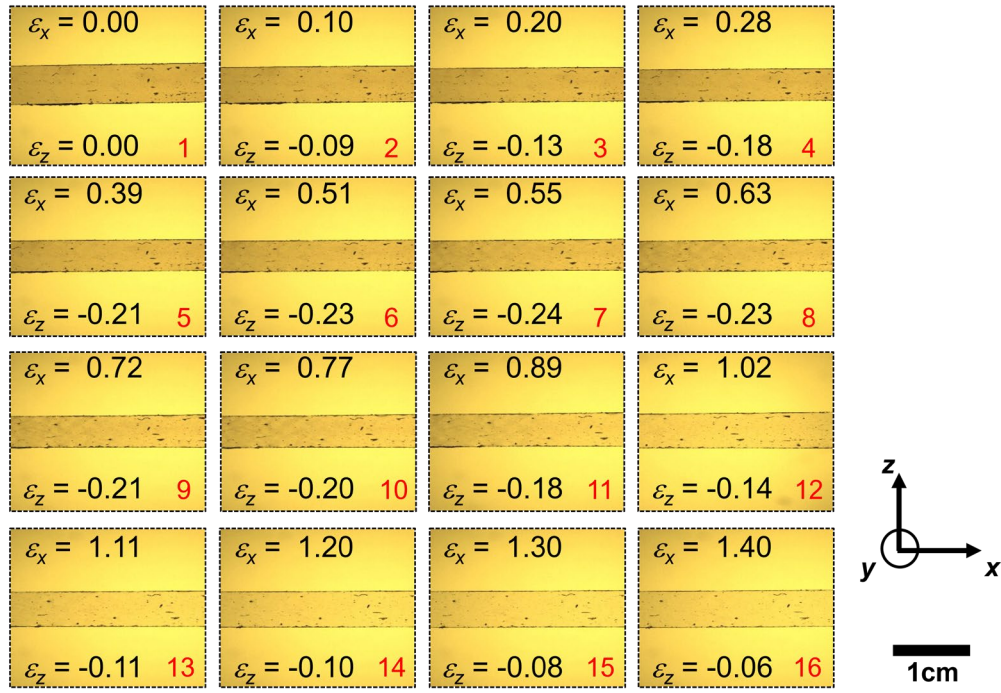
Figure 5.4 The whole mechanical deformation process of the H-LCE with photography displayed sequentially in increasing steps of \sim 0.1 strain. The scale bar is 1cm.
