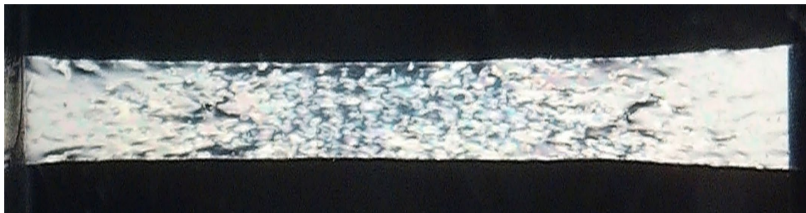
Figure 6.13 The non-uniform distribution of interference colours in non-dark regions indicates variations in the director alignment, resulting from deviations in the anticipated alignment profile during the deswelling process.
