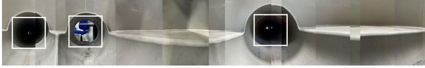
Figure 4.3: Template matching using NCC to identify exits.
