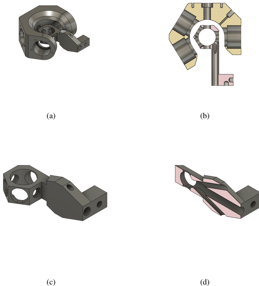
Figure 4.4: Model of two-part MPS design. Image (a) shows the claw and q-cell in the correct alignment for experimental work within the trap. (b): A top-down cross-section. (c): Q-cell only, shows circular cutouts over which glass coverslips were placed. (d): Cross-section along aerosol inlet (top), aerosol outlet (bottom) and relative humidity sensor port (the larger, central port).
