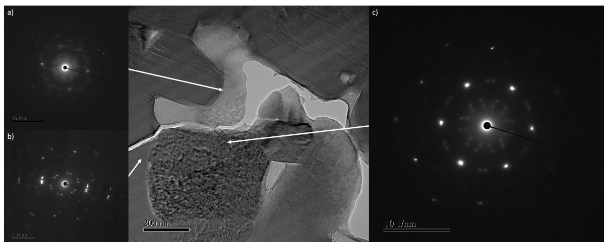
Figure 5.3: TEM micrograph of a bimodal pellet surface lamella (figure 5.2 d) with SEAD of three different areas.
