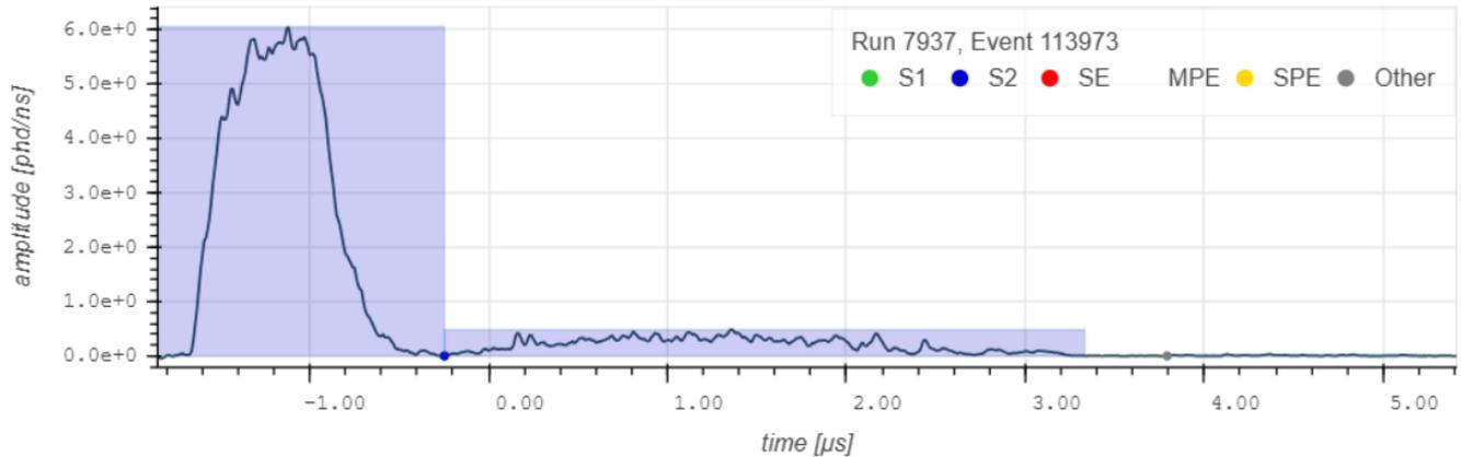
**Figure 6.14:** An example of the S2 pulses from a gate photoionisation event, where S2 light causes the emission of electrons from the gate grid.
